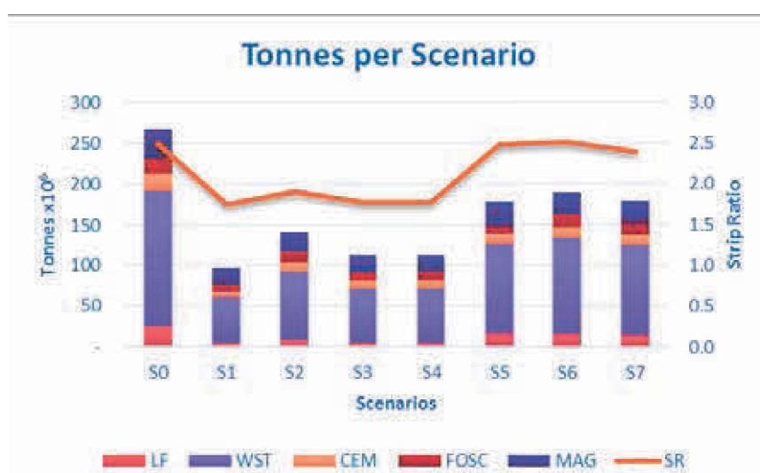
Figure 4 - Total tonnes per scenario and the respective proportion of tonnes of LF (landfill), WST (waste), CEM (cement), FOSC (phoscalcium), MAG (magnesia), SR (strip ratio)
