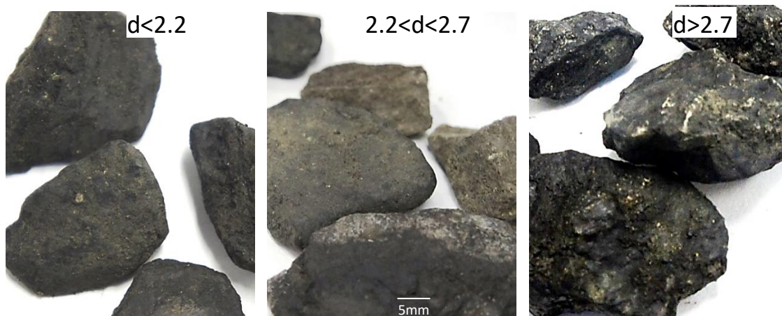
Figure 5. Images of the energetic fraction ( d < 2.2 ), intermediate fraction ( 2.2 < d < 2.7 ), and pyrite rich fraction ( d > 2.7 ) of the Bonito seam obtained after densimetric separation.
