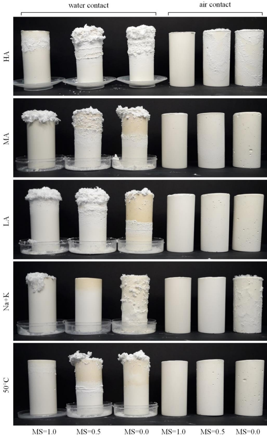
Figura 33 – Images of efflorescence of geopolymer samples after 28 days of either partial immersion in water or exposure to ambient air. HA= 25% Na 2 O, MA= 20% Na 2 O, LA= 15% Na 2 O, Na+K=20% Na 2 O+K 2 O, 50°C= 20% Na 2 O + curing at 50°C.
