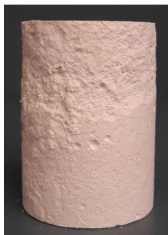
Fig. 16 – Sample with calcined kaolin as precursor and activated with 10% of \text{Na}_2\text{O} from NaOH with visible surface deterioration
