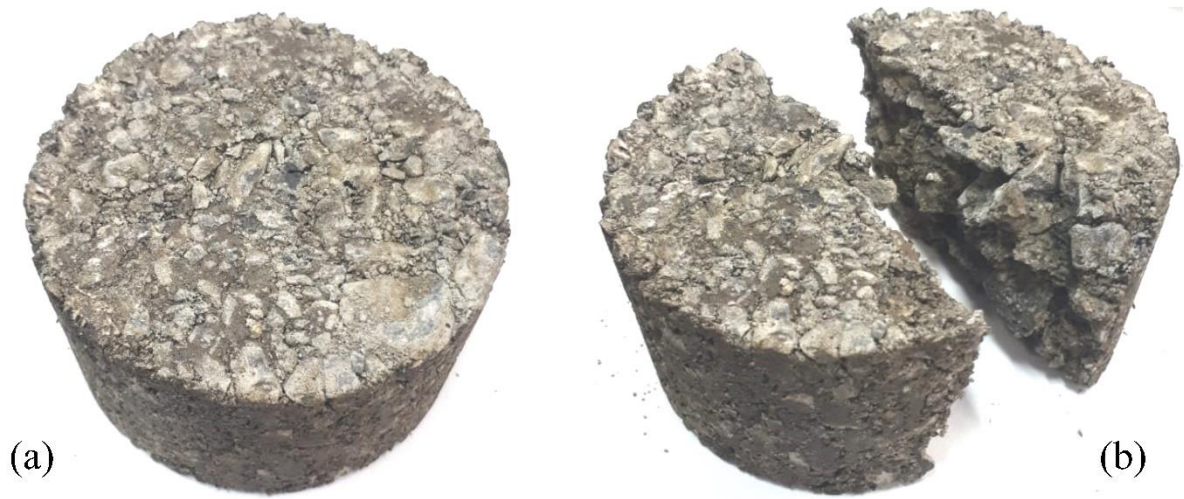
Figure 3. Specimen of cold recycled cement-treated mixture: (a) before and (b) after ITS test
