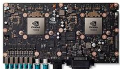
NVIDIA DRIVE™ PX is a powerful auto-pilot car computer designed to run the deep neural networks that will enable a car to see, think, and learn.
