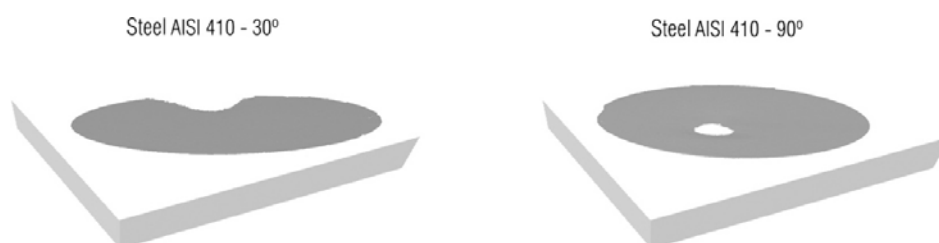
Figure 8. Three-dimensional scanning of the samples submitted to the jet slurry erosion test.
