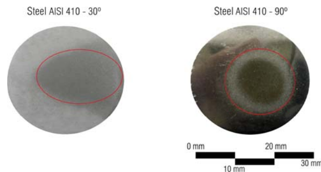
Figure 7. Areas of the eroded regions of the materials submitted to the jet slurry erosion test.
