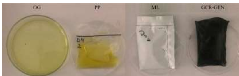
SUPPLEMENTARY FIGURE 1 Visual aspect of extra-virgin olive oil packed in open dish glass (OG), polypropylene film (PP), Al-laminated (ML) and genipin crosslinked film (GCR-GEN).
