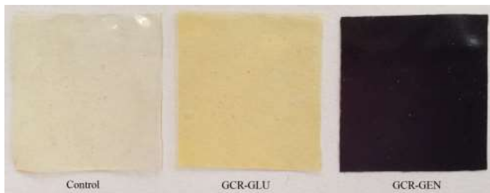
FIGURE 3 Visual appearance of the control film and films crosslinked with glutaraldehyde (GCR-GLU) and genipin (GCR-GEN).
