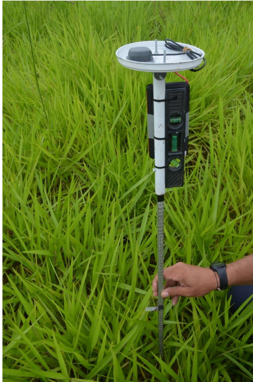
Figure 3: Sward stick coupled to a RTK-GPS.
