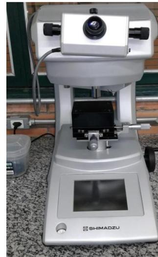
(b) Microdurômetro SHIMADZU HMV-G 20ST
