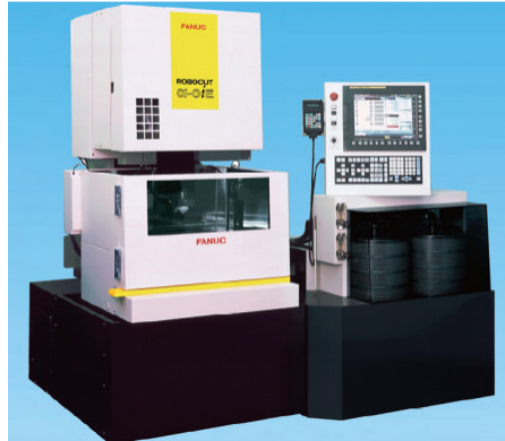
Figure 9 – Equipment used for wire electroerosion cutting [10].
