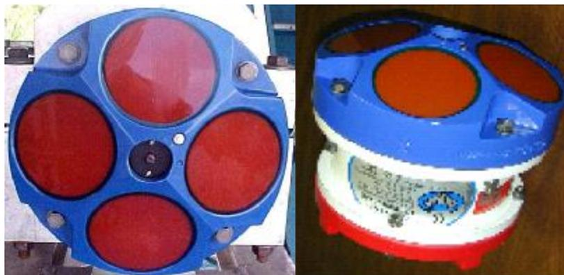
Figura 4.3 – ADCP de 1200 KHz
