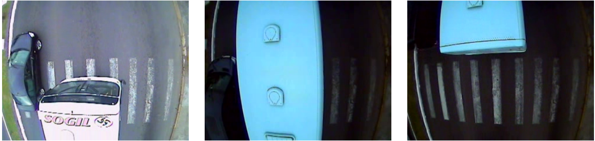
Figure 4.2: Example of the changes in camera gain caused by the buses passing through the virtual loop too close to the camera (top view).
