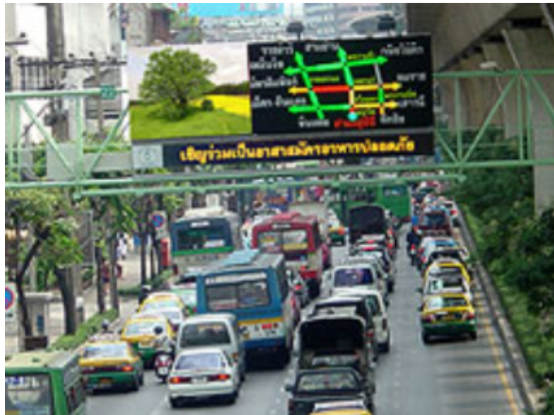
Figure 1.1: Genius traffic system, in Thailand. The system indicates in real-time which streets may have traffic jams, allowing drivers to change their route and improving the traffic flow.
