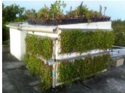
Figure 3.23: Green walls added to the former prototype analysed by Wilkinson & Feitosa (2015). (Source: Wilkinson et al., 2017)
