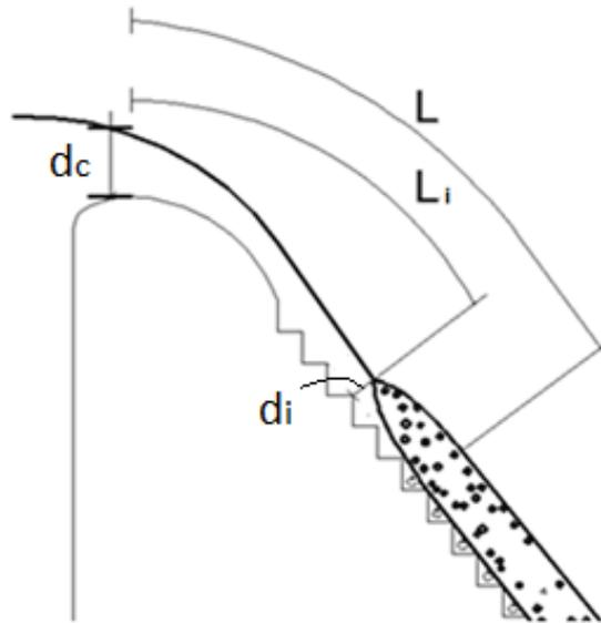
Figure 1 – Scheme of the main flow characteristics used for the normalization of the pressure head along the chute.
