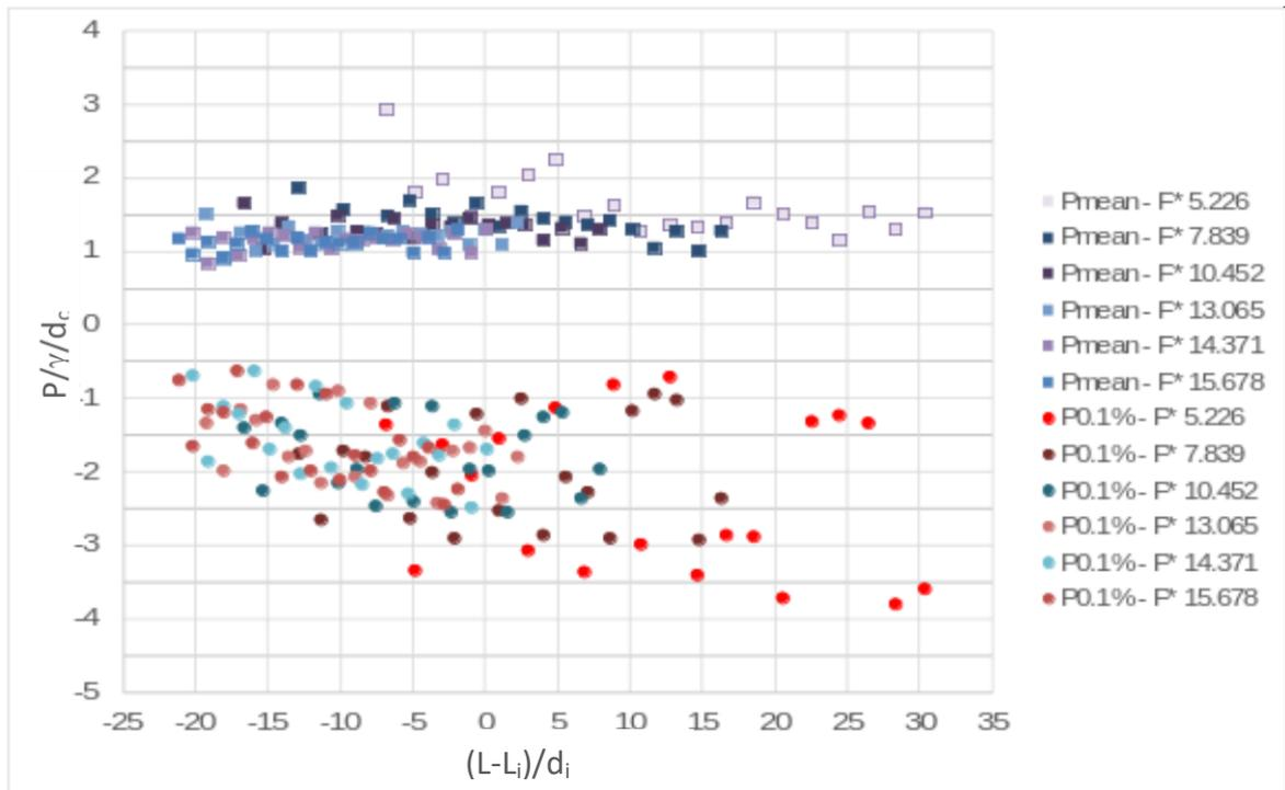
Figure 2 – Mean and extreme pressures ( $P_{0.1\%}$ ) acting on the horizontal faces of the steps, in the vicinity of their edges.
