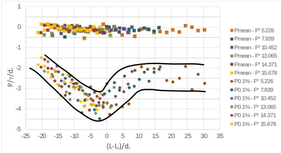
Figure 3 – Mean and extreme pressures ( $P_{0.1\%}$ ) acting on the vertical faces of the steps, in the vicinity of their edges.
