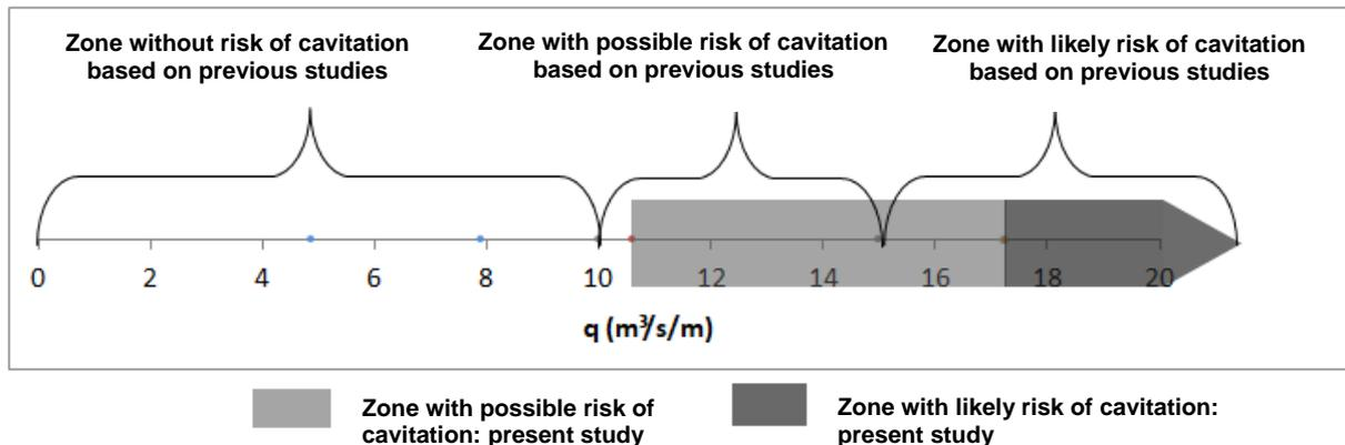
Figure 4 - Limit flow rates regarding the tendency of cavitation on steeply sloping stepped spillways, based on critical extreme pressure data with a very low probability of non-exceedance, in the vicinity of the point of inception: comparison with other studies.
