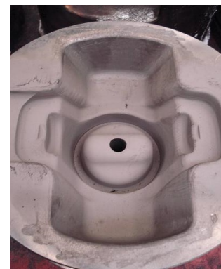
Fig. 5 The bottom die used for forging, finished with manual grinding and then thermal spray coated.
