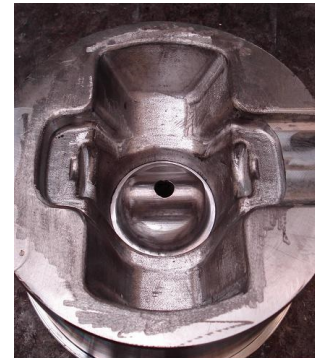
Fig. 4 The bottom die used for forging, finished with manual grinding.
