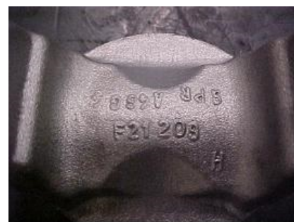
Fig. 11 Photo of one of the last parts of the coated die batch.
