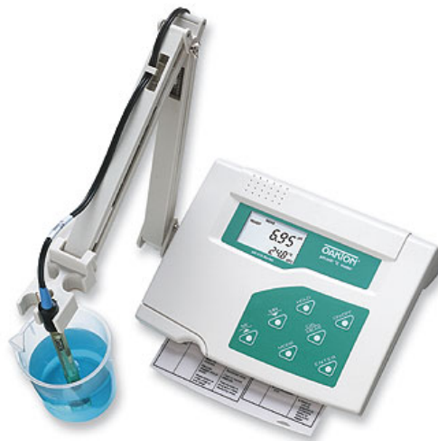
Figure 4.8: Oakton pH 510 benchtop meter and all in one Ag/AgCl reference electrode packaged along the sensing electrode and temperature sensor.
