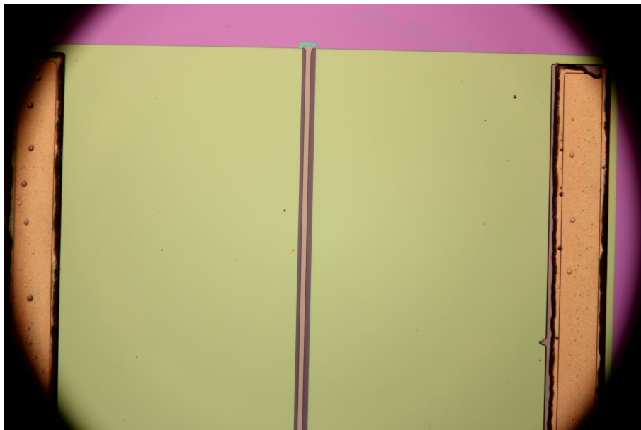
Figure 5.11: Channel oxide exposed after the gate etching and the source/ drain contacts covered with photoresist.
