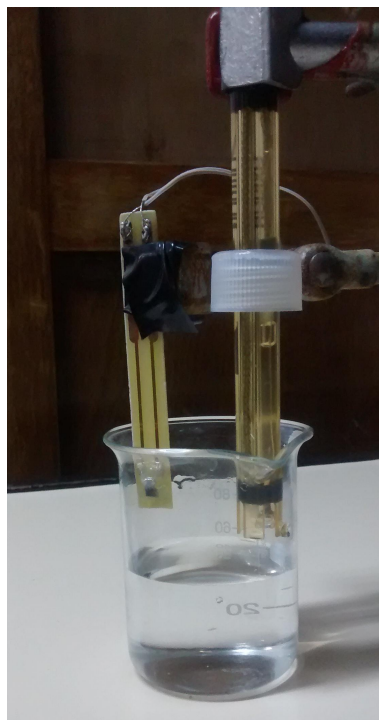
Figure 7.1: ISFET experiment picture. With the use of a "claw" support the sensor and the reference electrode are placed into the aqueous solution and connected to the semiconductor parameter analyzer.
