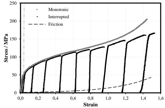
Fig. 6. Stress-strain data obtained from monotonic and interrupted tests.
