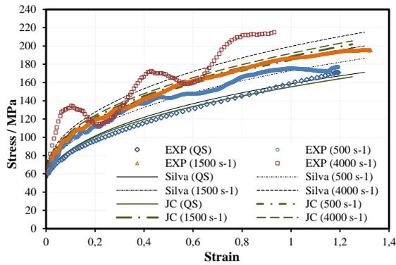
Fig. 5. Stress-strain data obtained from high strain-rate tests.
