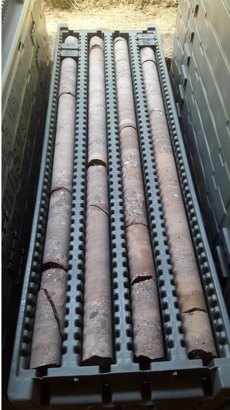
Figure 1.2: Example of a box containing a sequence of core samples labeled by depth.
