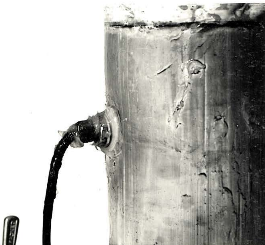
FIGURE 6.4 A - PICTURE OF THE MEMBRANE PROTECTION AND SILICONE RUBBER COMPOUND USED AS AN EXTRA PROTECTION
