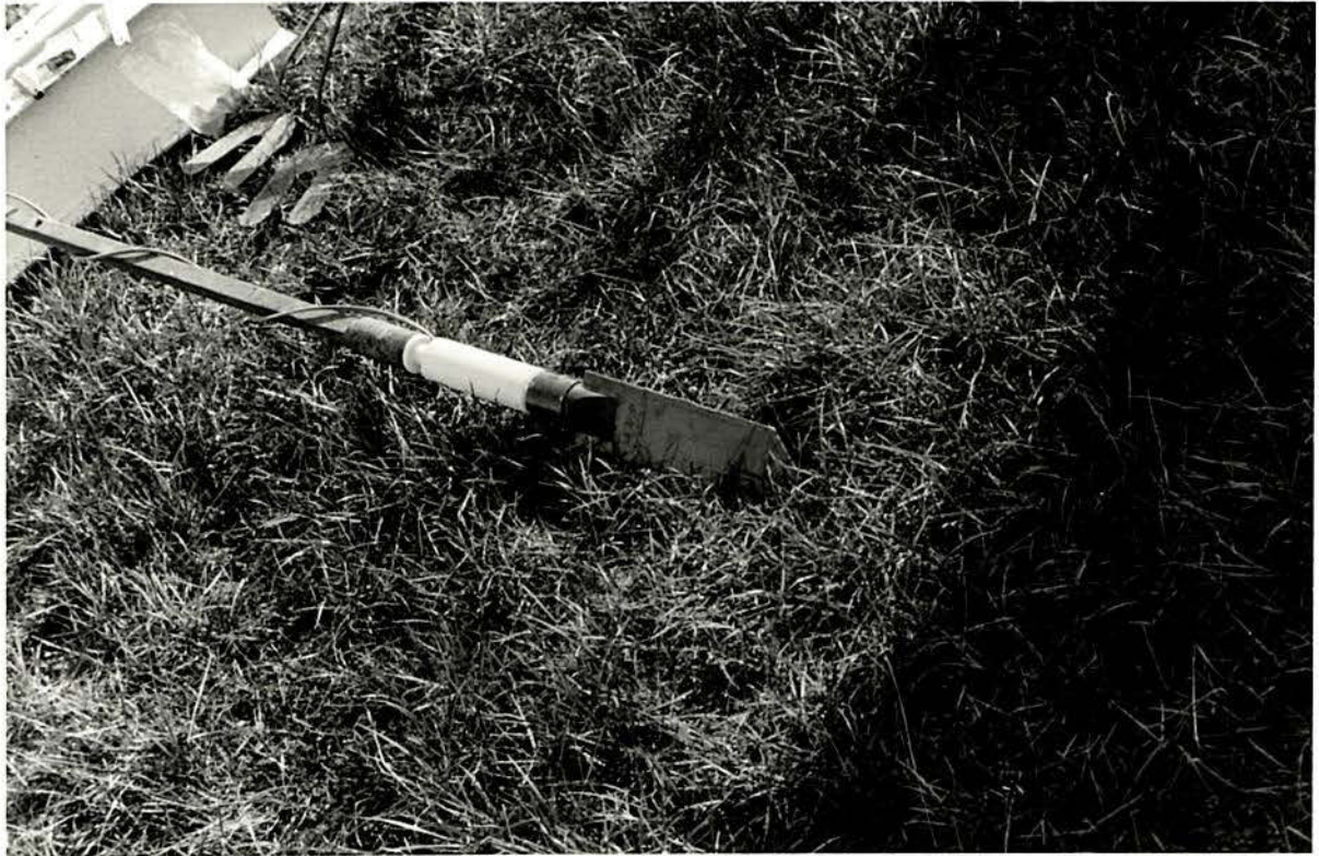
(A) "DRIVE IN" TOTAL STRESS CELL WITH ADAPTOR AND SPT RODS
