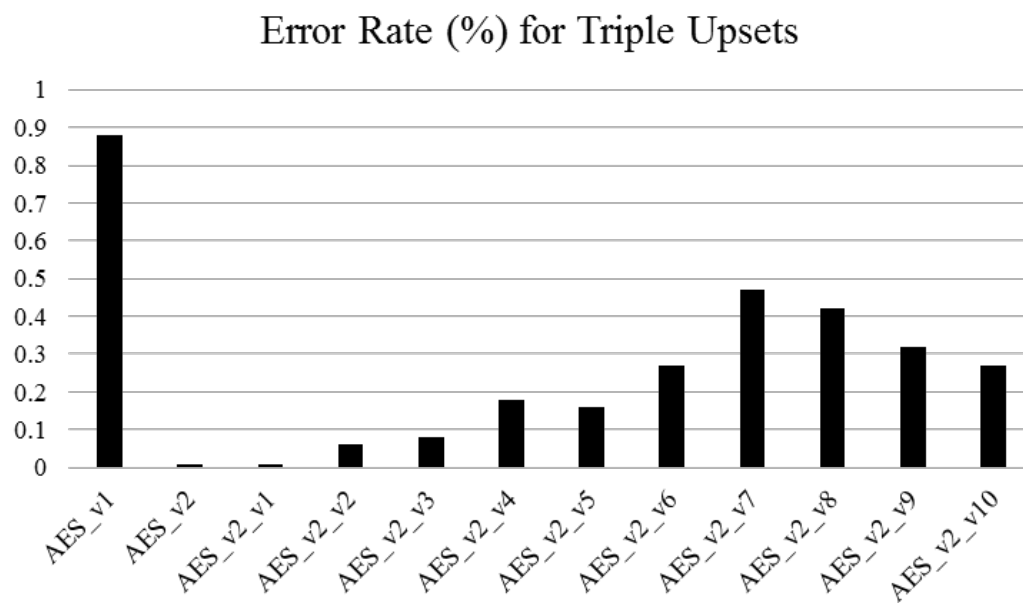
Fig. 41 Error rate for triple faults in TMR designs with different granularities
