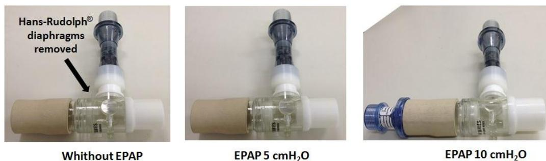
**Figure 1:** Experimental device applied to obtain different expiratory positive airway pressure (EPAP) intensities during exercise.
