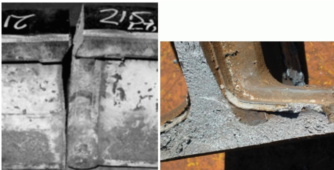
Figura 2.28 – Fratura Transversal (MUTTON, 2004) e (DUVEL, 2005).
