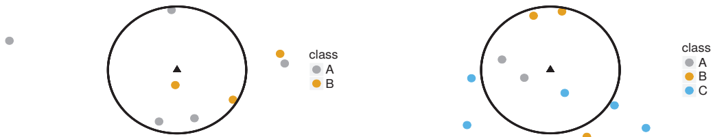
Figure 3.2 At left a binary classification problem and the query point (triangle) and its 5-neighborhood. At right a multiclass problem and the query point (triangle) and its 5-neighborhood.
