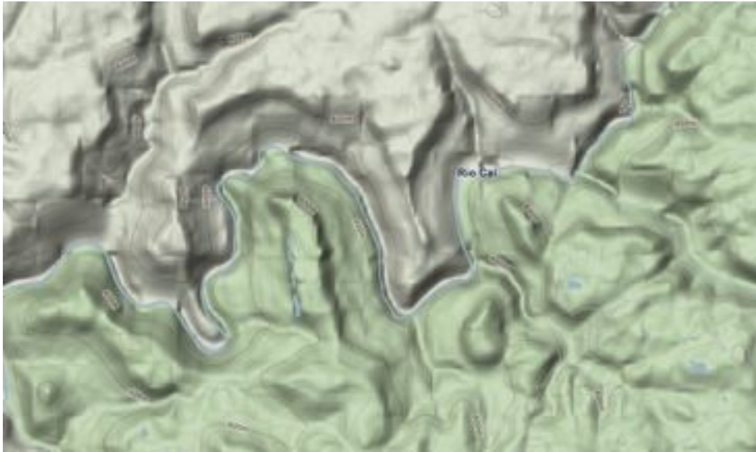
Figure 1.1: Cartography contour lines. Isocontours represent different elevations on the terrain. Each line has one height associated. With this visualization technique, it is much easier to understand the position of peaks and depressions in the terrain. In this particular image, the relief shading helps the visualization even further. Image extracted from Google Maps®.
