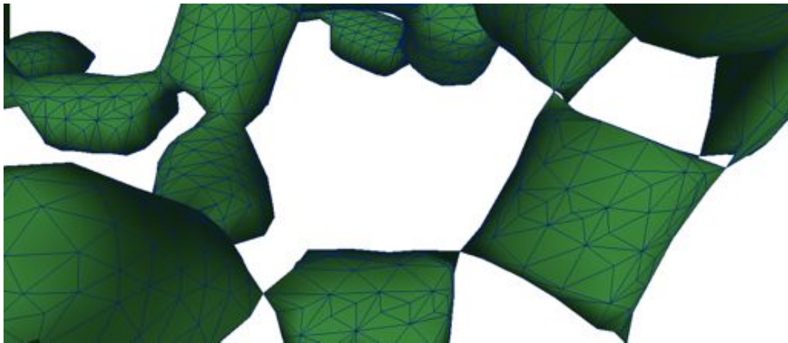
Figure 2.4: Non manifold triangular mesh. The surface has vertices that are shared by distinct parts, and locally are not topologically equivalent to a disk.
