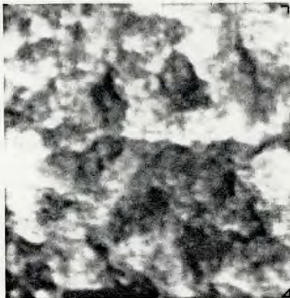
Fig. 4. SEM image of the surface of the Fe-Al bilayered sample annealed at 650 K. (Magnification, 10 000 \times .)
