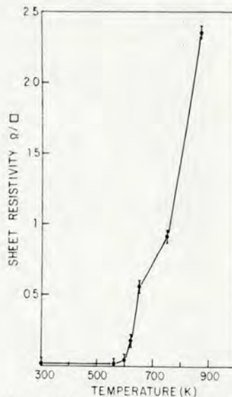
Fig. 9. Sheet resistivities of Fe–Al bilayered samples subjected to isochronous anneals for 60 min at temperatures between 300 and 870 K
