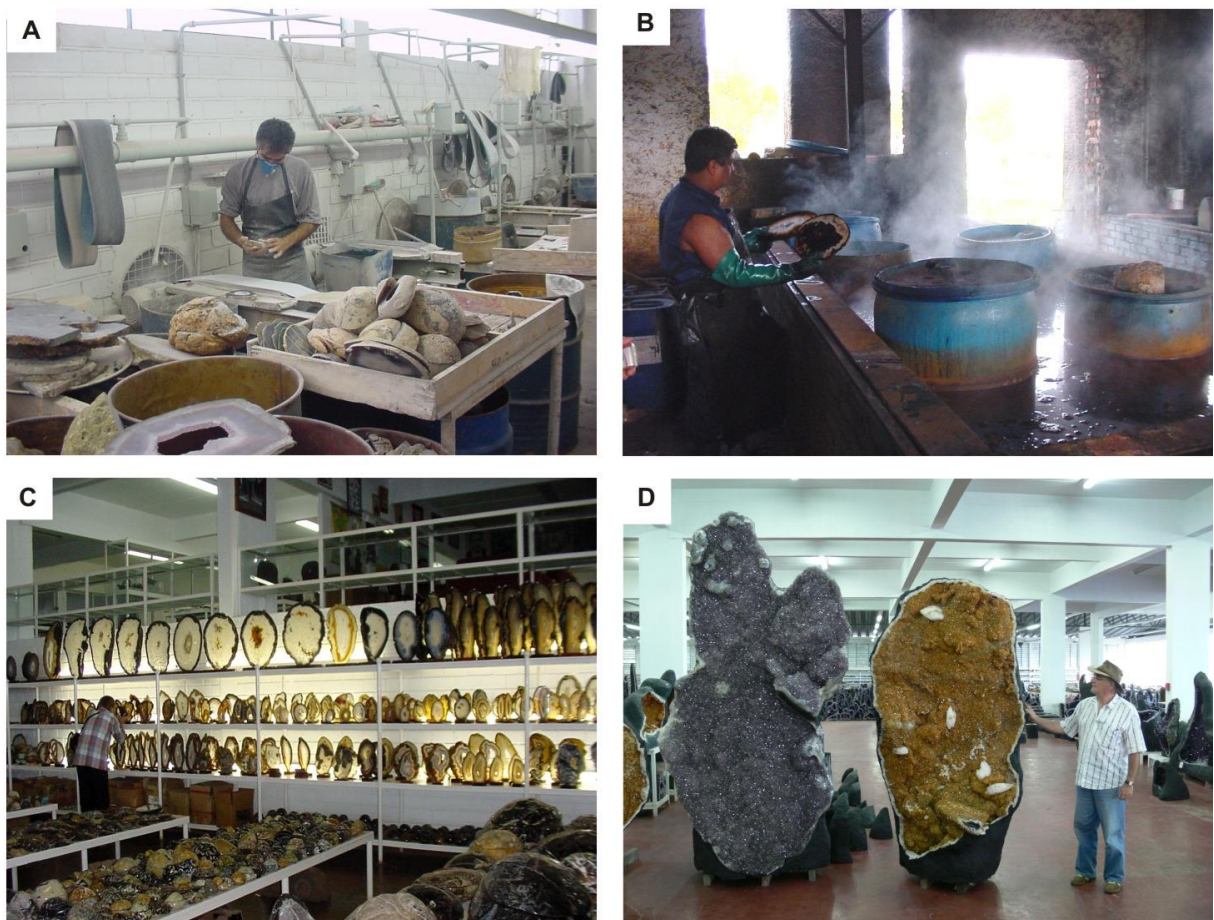
Figure 11 - Gem processing and gemstones workshop in Soledade A – Polishing agate geodes and agate plates. B – Dying agate geodes and plates. C – Exposition of polished agate plates. D – Geode pieces filled with amethyst, citrine (heat treated amethyst) and calcite crystals.
