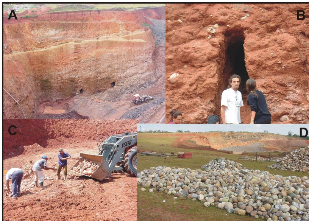
Figure 4 – Surface agate mining in Salto do Jacuí Mining District. A and B – open pits and underground adits opened in the weathered volcanic rock. C – miners collecting agate geodes in the removal regolith. D – agate geodes to be commercially classified; in the back, the surface mine.
