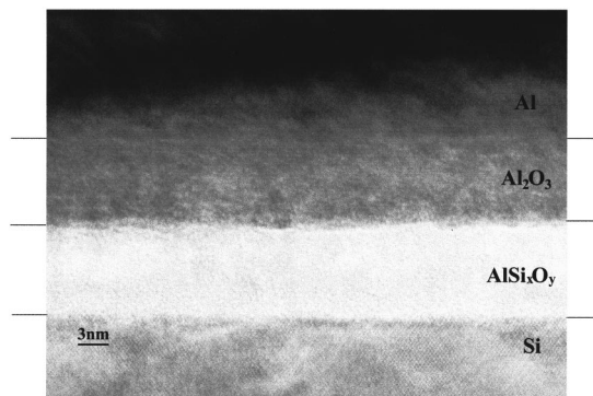
FIG. 3. TEM image \text{Al}_2\text{O}_3 deposited on silicon at \sim 400 °C in the as-deposited state. The total film thickness is approximately 18 nm. Two distinct layers are observed with approximately equal thickness.
