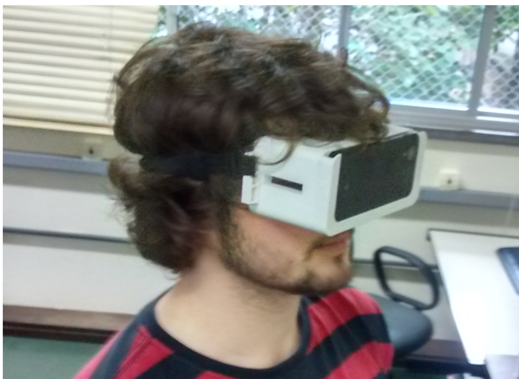
Plastic 3D printed HMD case (white) with a Nexus 5 phone (black) inside.
