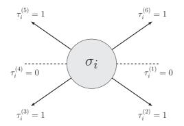
FIG. 1. The occupational and orientational states of a molecule at the site *i*. The arms variables are:  $\tau_i^{(1)} = 0$ ,  $\tau_i^{(2)} = 1$ ,  $\tau_i^{(3)} = 1$ ,  $\tau_i^{(4)} = 0$ ,  $\tau_i^{(5)} = 1$ ,  $\tau_i^{(6)} = 1$ .
