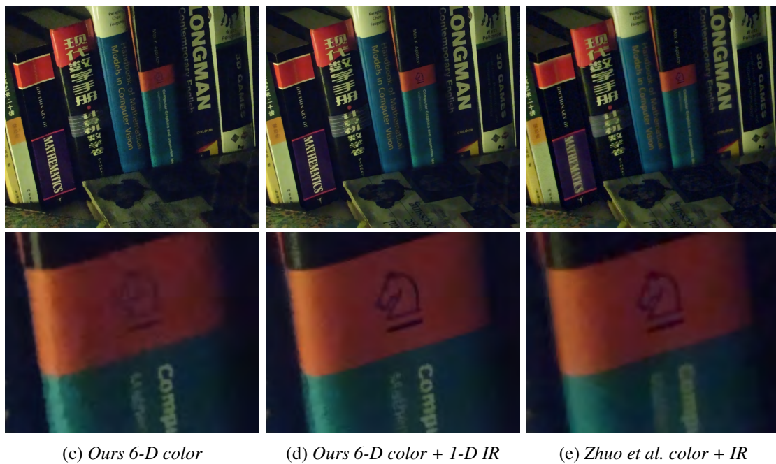
Figure 4.16: Example of denoising using additional information from an infrared-color image pair (a) and (b). Using non-local-means on the color data ( 7 \times 7 -pixel patches, reduced to 6-D) reduces noise but introduces blur (c). By using the infrared data as an extra dimension, our filter achieves optimal denoising for the scene (d). The original algorithm of Zhuo et al. (ZHUO et al., 2010) uses a geodesic filter for denoising, which does not work effectively for higher dimensions. Their result exhibits blurring in regions such as in the text on back of the books (e).
