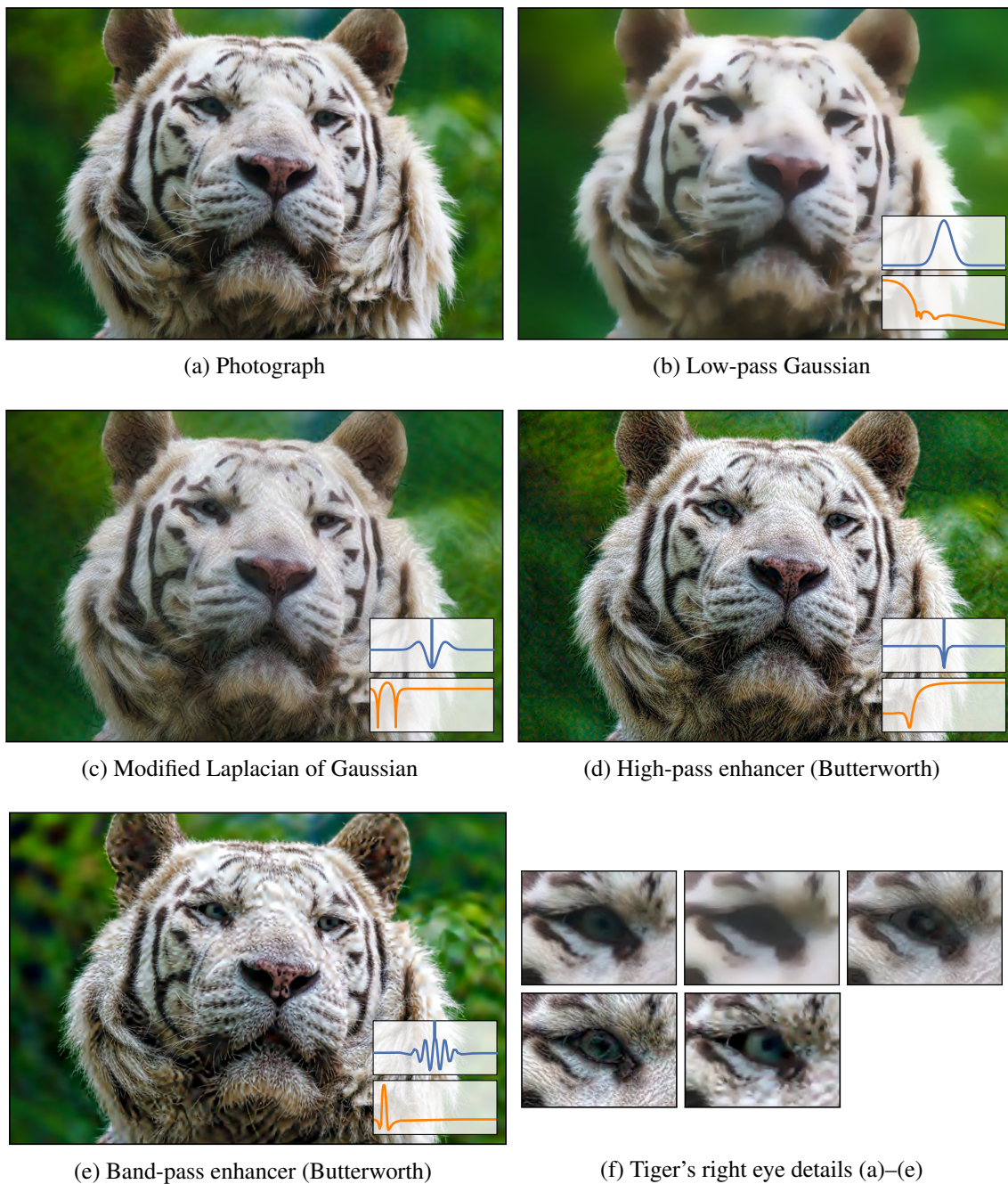
Figure 5.1: A variety of high-order recursive filters applied by our method to the photograph in (a). For these examples, non-uniform sampling positions are computed using an edge-aware transform. Thus, the resulting filters preserve the image structure and do not introduce visual artifacts such as halos around objects. The graphs in the insets show the filter's impulse response in blue, and its frequency response (Bode magnitude plot) in orange.
