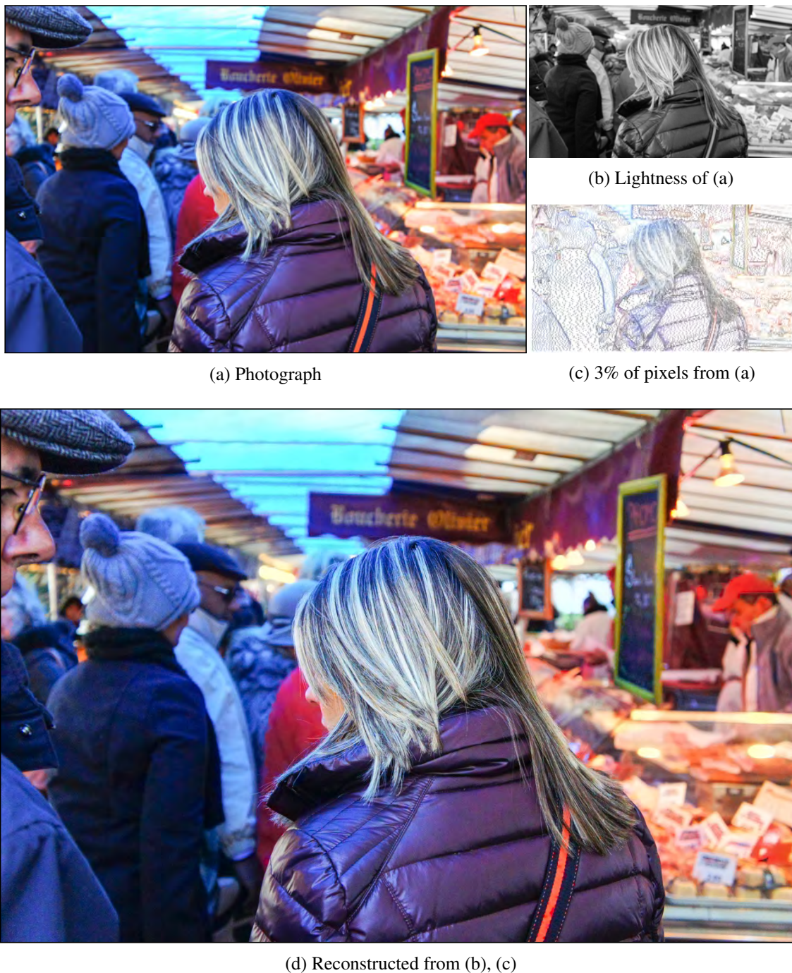
Figure 5.11: Example of data-aware interpolation using non-uniform filtering. A full-color image is reconstructed from the lightness channel and only 3% of the pixels from the original image, shown in (a). The pixels in (c) were importance-sampled using the gradient magnitude of the lightness channel. PSNR of (d) vs (a) is 31.17 dB.
