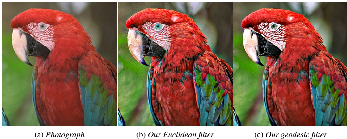
Figure 2.2: Example of color detail enhancement using our geodesic and Euclidean filters: the Domain Transform (Chapter 3) and the Adaptive Manifolds (Chapter 4), respectively. Each filter enhances image features differently: note the colors of the parrot’s eye. The Euclidean filter generates a result in between global and local contrast enhancement, while the result of the geodesic filter is mostly local. Choosing between the two results is a subjective choice.
