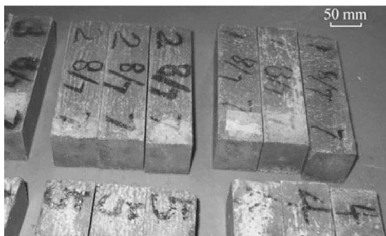
Figure 5 Bricks made using recovered nonmetallic PCB material. Source: Mou et al. (2007).
