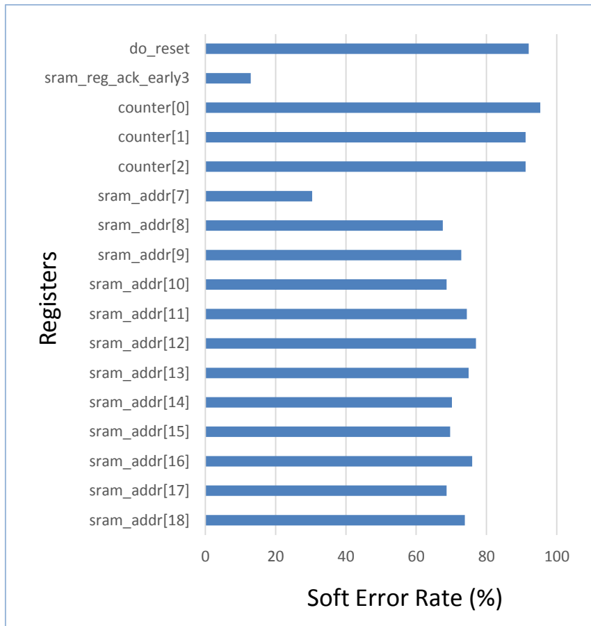
Figure 5.10 Soft error rate due to SET in the clock tree network.
