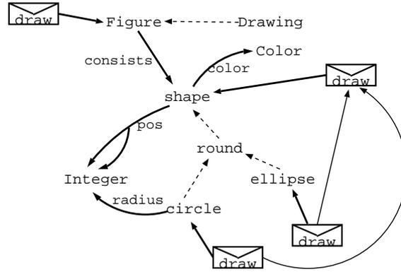
Figure 2.3: Class-model graph for geometric figures
