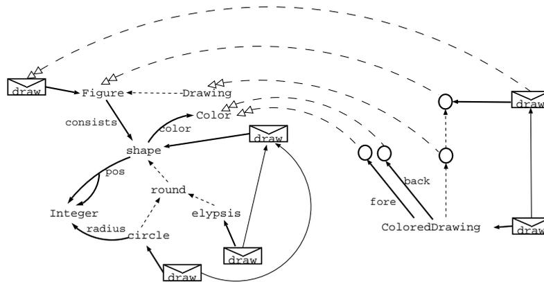
Figure 2.7: Specialization through inheritance as class-model graph composition
