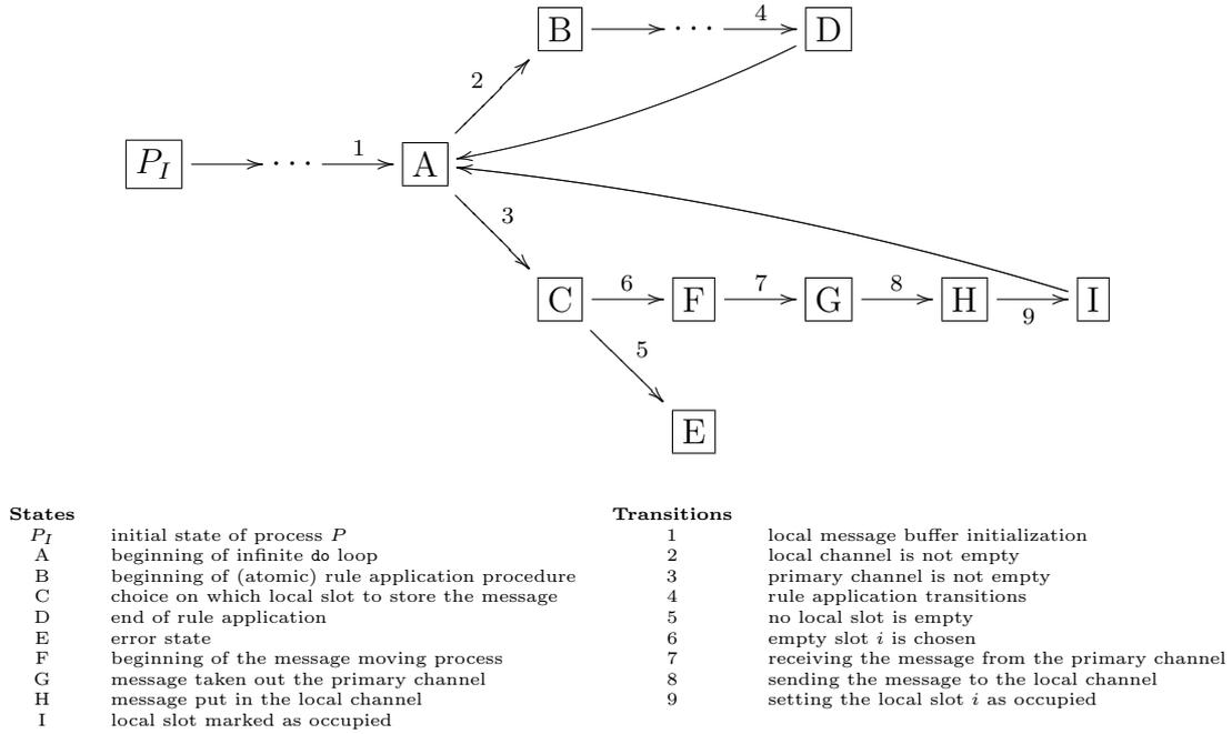
Figure 4.6: Object process transition system
