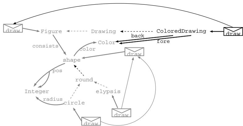
Figure 2.8: Specialization through inheritance as class-model graph composition
