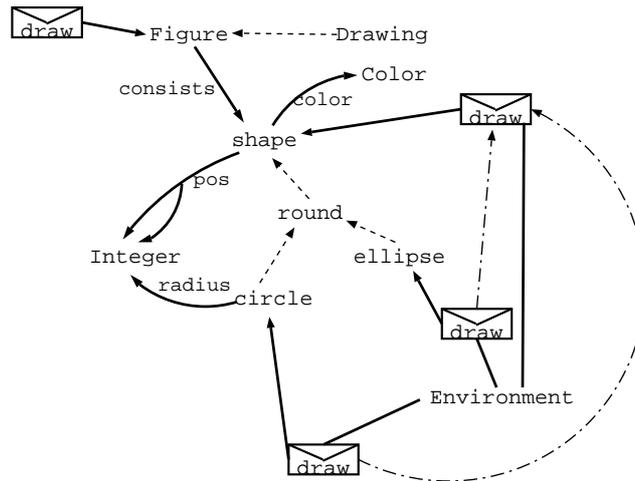
Figure 2.4: Class-model graph for geometric shapes
