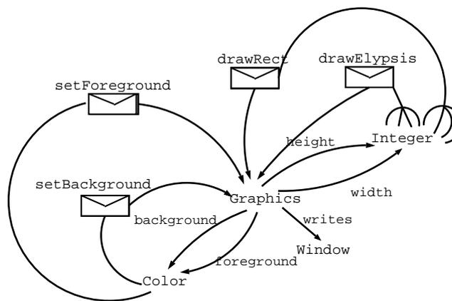
Figure 2.5: Class-model graph for graphic primitives
