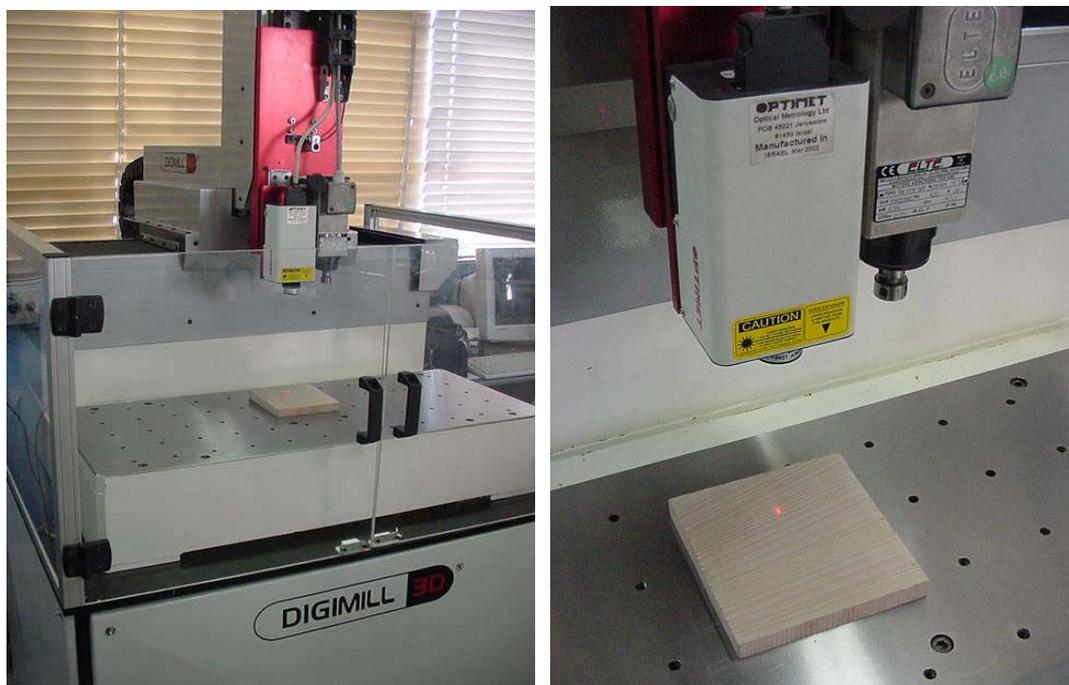
**Figura 64 - Scanner Tridimensional a Laser modelo Digimill 3D.**
