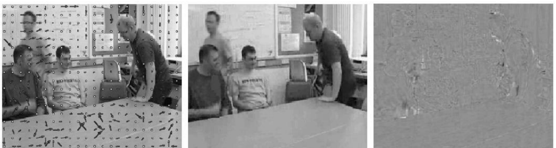
Figure 2: Motion vectors over the frame, frame n compensated and associated residual frame, respectively. Source: (Richardson 2011)
