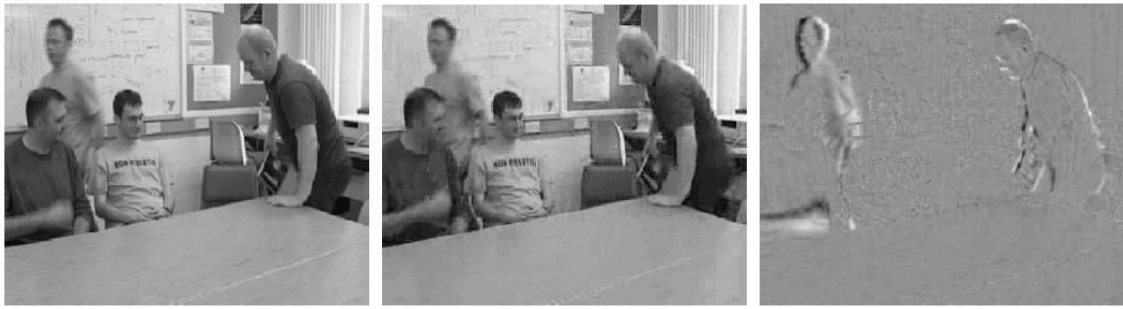
Figure 43: Frame n to encode, Frame n-1 (reconstructed after encoding), and associated residual frame, respectively. Source: [7]
