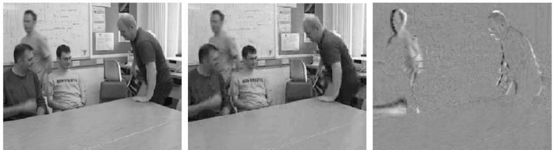
Figure 1: Frame n to encode, Frame n-1 (reconstructed after encoding), and associated residual frame, respectively. Source: (Richardson 2011)
