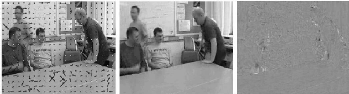
Figure 44: Motion vectors over the frame, frame n compensated and associated residual frame, respectively. Source: [7]
