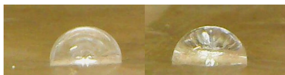
Figure 1. Images of droplets formed on G/A films at pH 5 and 7 (from left to right)
