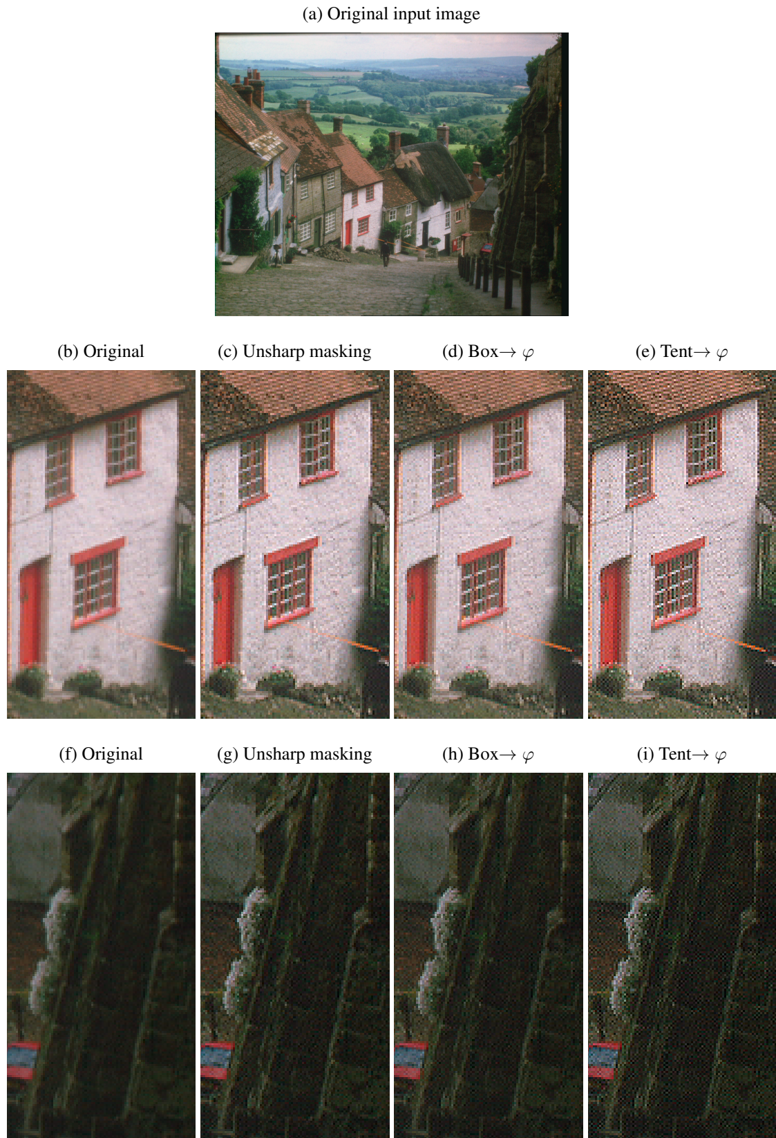
Figure 5.3: Natural image enhanced with regular unsharp masking (with \sigma = 1 and gain 0.5), Box and Tent. Notice how Box achieves good results without the need for parameter tweaking.
