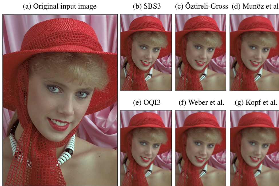
Figure 5.5: Downscaling by a factor of 5 (to a size of 103 \times 154 ). Note how details of the hat and scarf, as well as the face and eyes, are better outlined due to SBS3's sharpness. (These images are better seen in the supplementary materials to avoid the unwanted resampling done by the PDF reader).
