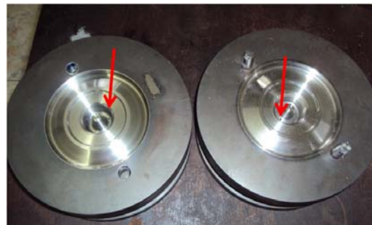
Fig. 14 The holes to facilitate the exit of air.
