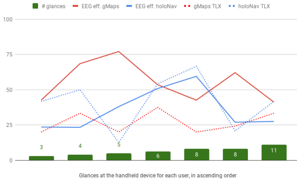
Figure 4.4: Observed number of glances at the handheld device, EEG efficiency and NASA TLX results for each subject.
