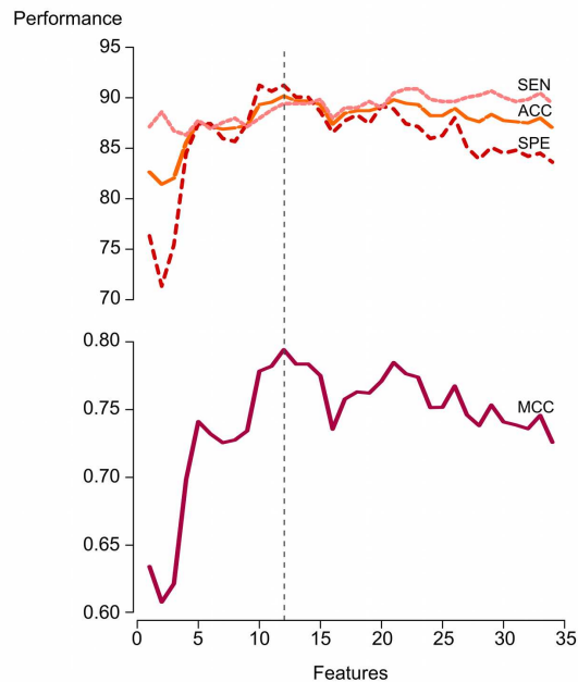
Figure A.3: Performance of the RF model evaluated by means of a restricted forward feature selection. The best and most balanced performance in terms of sensitivity and specificity is achieved by the model trained based on the subset of top 12 features.
