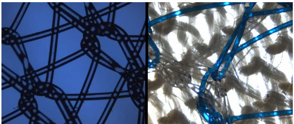
Fig 1. Macroscopy of the polypropylene mesh (left) and the coated polypropylene mesh (right) with a six cm 2 area.
