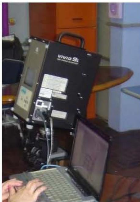
Figura 40: scanner Vivid 9i Konica Minolta
