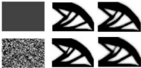
Figure 3. Non convexity of the objective function, Eq. (16), for exponent 1/8 and different initial density distributions.
