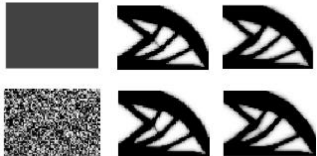
Figure 4. Results obtained with the continuation approach. The first column shows the initial density distributions, the second row shows the results obtained with the IWSF filter and the third column shows the results obtained with the AWSF filter.
