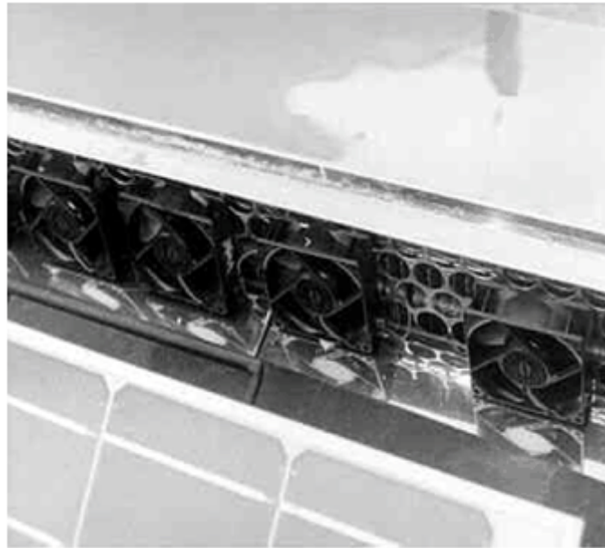
Figure 4. Fans placed close to the evaporator.
