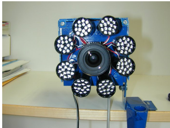
Figure 62 – IDS uEye UI1210-C Camera Equipped with Infrared Flash Strobes
