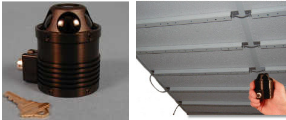
Figure 11 – HiBall Sensor (left) and Ceiling Equipped with Beacon Array Modules of HiBall 3100 System (right)
