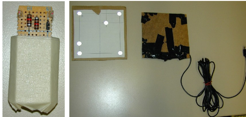
Figure 64 – Active Marker Prototypes: 2-marker Non-tethered Label (left); Passive and Equivalent Active Marker Tethered Label for PTrack (right)
