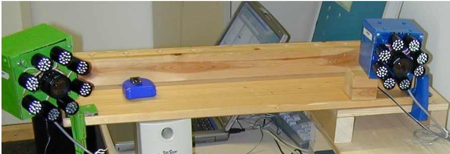
Figure 99 – View of both Cameras in PTrack Multiple-camera Configuration
