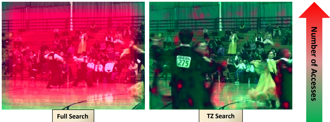
Figure B.5: Output Exapmle: reference frame access index considering two block matching algorithms: Full Search and TZ Search.
