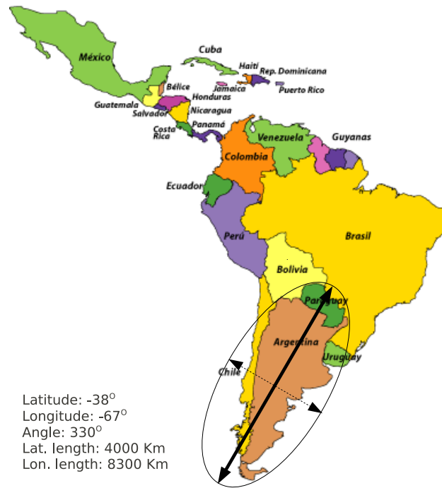
Figure 5.1: Mesh refinement area definition of a specific region of the Earth. In this example, parameters were determined for an ellipse area to cover Argentina.
