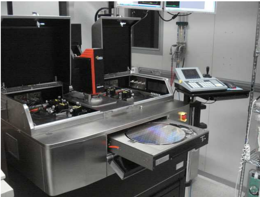
Figure D.2: Probe Station Suss Wafer Prober PB300 consisting basically of micro-manipulators, shielding, wafer chamber and chuck, and joystick controller.
