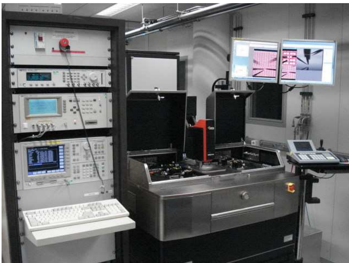
Figure D.1: Measurement System consisting basically of an HP4156, an HP4284, a probe station Suss Wafer Prober PB300, and software applications (IMEC – Belgium).
