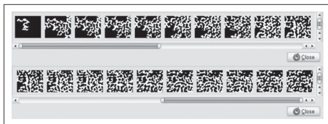
Figure 4. Display of the connectivity propagation for a single throat along the slices.
